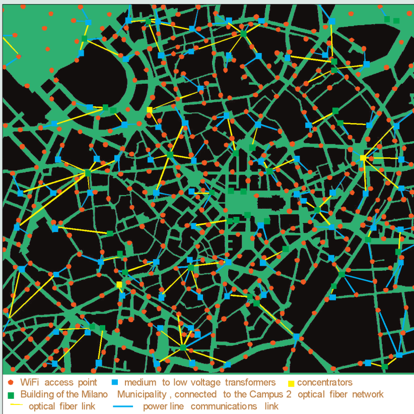
■ Figure 2. Planning of the radio coverage and backhauling of the central area of Milan (about 5 km 2 ).
